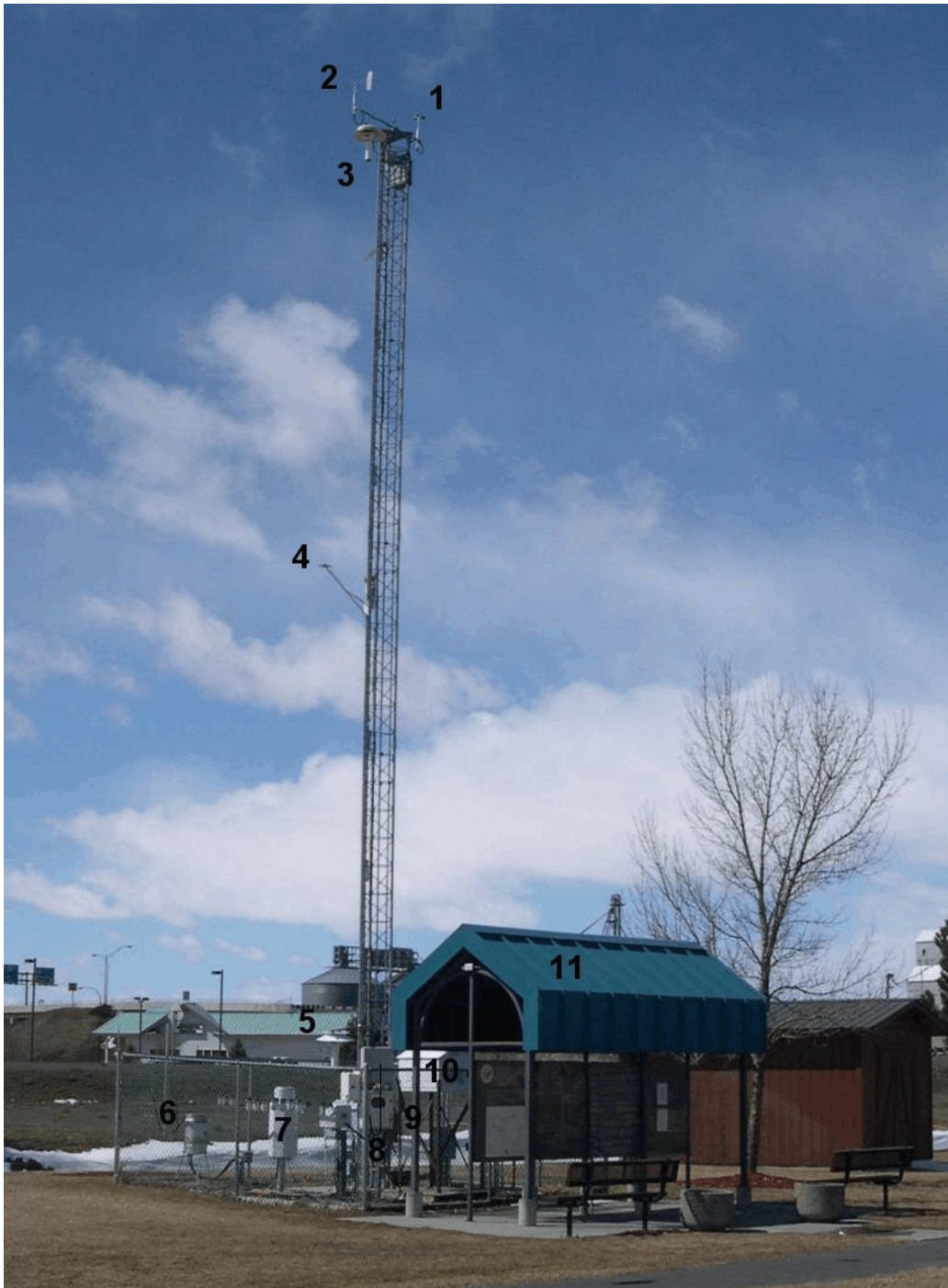
Figure F-1. Example NOAA INL Mesonet station layout, with the addition of the community monitoring station kiosk (foreground) on the Idaho Falls Greenbelt at the John's Hole Bridge and Forebay.
